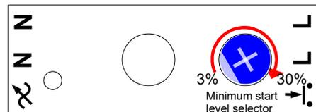
Warning: all LED type lamps have a minimal start-up tension, this tension could be higher than the minimal dimmable value. After setting this minimal value with the regulation selector , you have to dim the lamp to his lowest intensity with the push button ( long push ). Stop and start again your lamp with a short push . IF the lamp doesn't start up lighting then start again all the procedure and increase with the selector the minimal value .
